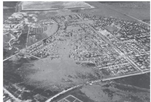
Figure 17. The Merriespruit tailings dam failure of 1994, with destruction of the village (Fourie & Papageorgiou 2001).
