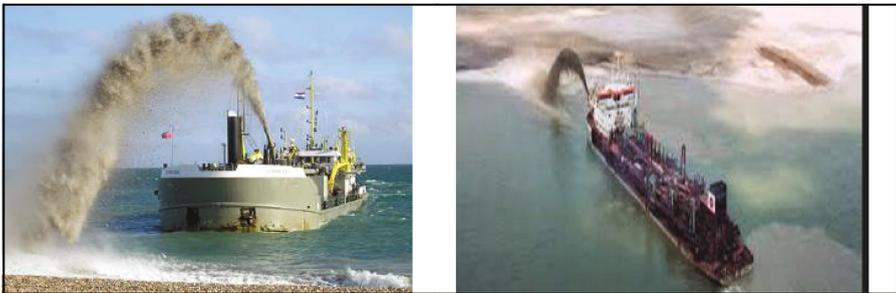
**Fig. 3.** Typical photos of sand dredging operations
