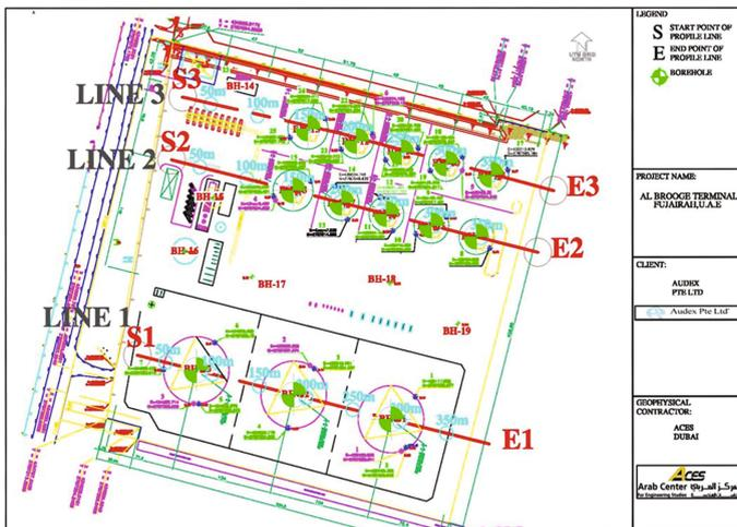
Fig. 23. Layout of 3 MASW lines covering all tanks locations
