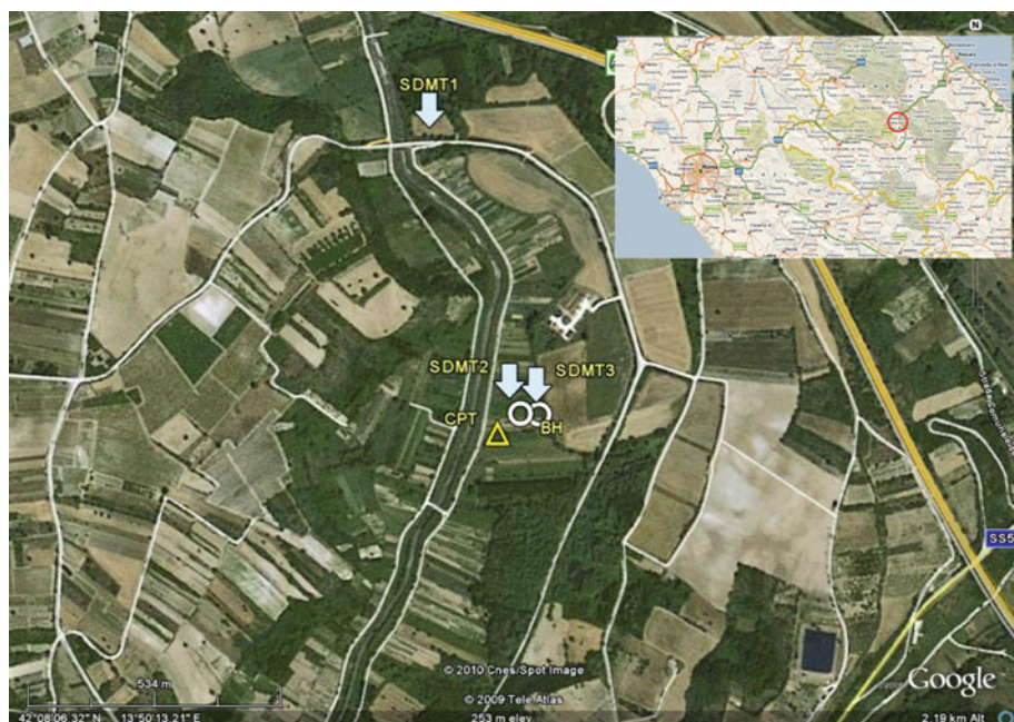
Fig. 9 Location of tests in the area of Vittorito to analyse the occurrence of liquefaction (BH = borehole; SDMT = seismic dilatometer test; CPT = cone penetration test)
