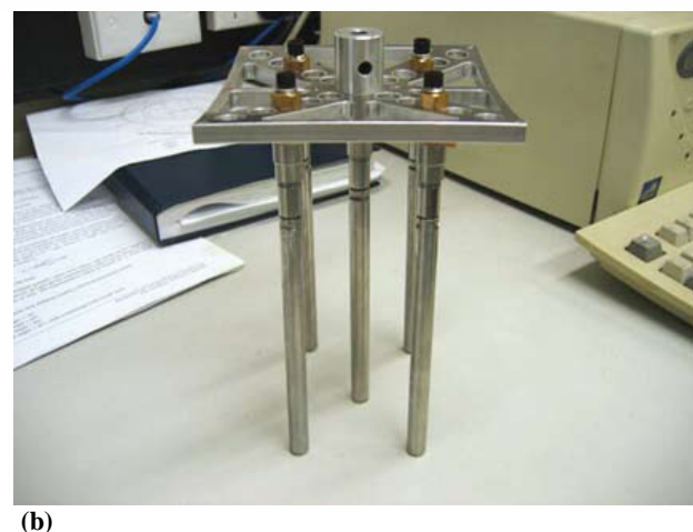
Figure 3.15. Installation of piles; a) influence of methods, in-flight or at ng on pile normalized lateral pressure p\gamma/d with \gamma unit weight and d pile diameter (Dyson & Randolph 2001); b) pile group (Gaudin & Lehané 2006).
