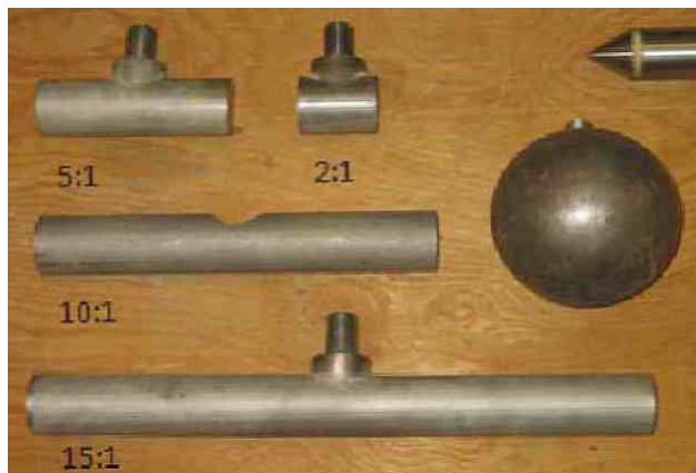
Figure 4.32. Full-flow penetrometers including the ball-penetrometer and various T-bars for strength testing of very soft offshore soils (Yafate et al. 2007).
