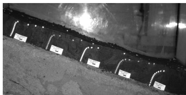
Figure 3.29. Soil movement shown by markers after 1 thawing cycle of thawing (Harris et al. 2008).
