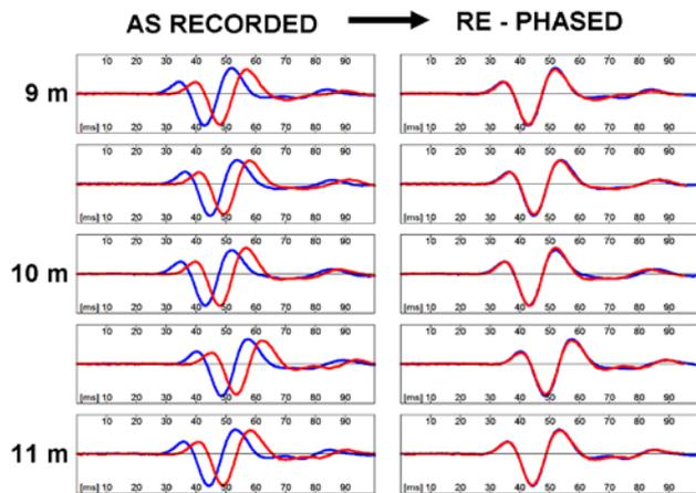
Figure 2. Example of seismograms obtained by SDMT at the research site of Fucino (Italy)
