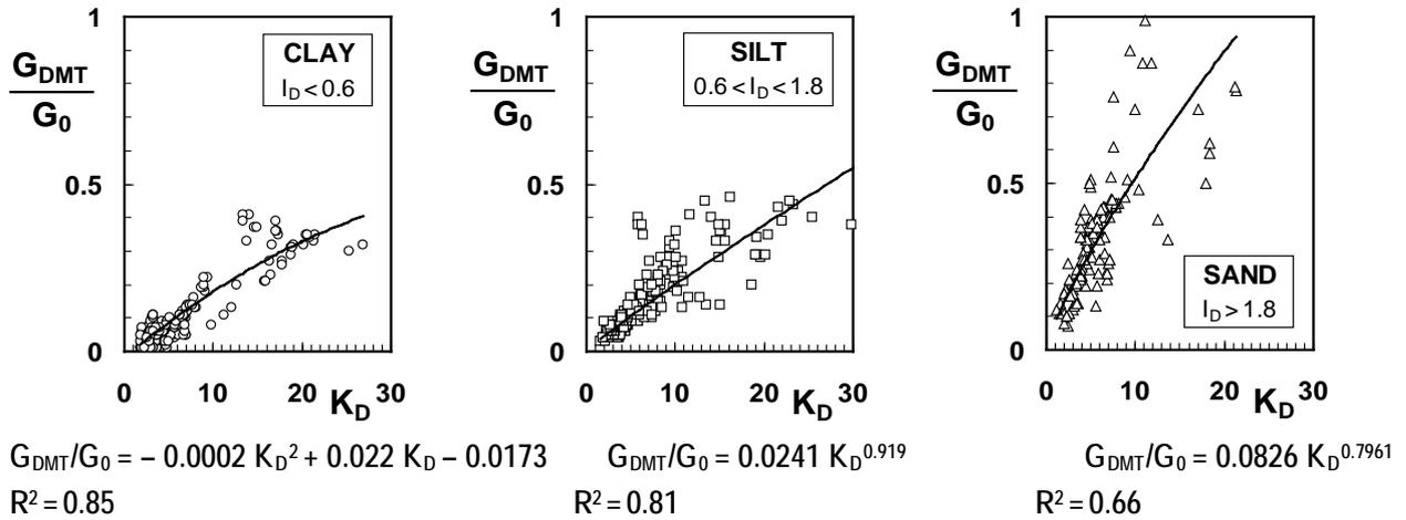
Figure 7. Decay ratio  $G_{DMT}/G_0$  vs.  $K_D$  for clay, silt and sand (Marchetti et al. 2008)
