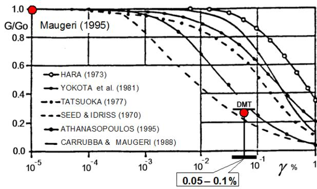
Figure 5. Tentative method for deriving  $G$ - $\gamma$  curves from SDMT
