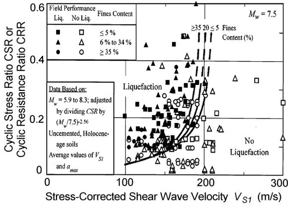
Figure 9. Curves for evaluating CRR from  $V_S$  for clean uncemented soils (Andrus & Stokoe 2000)
