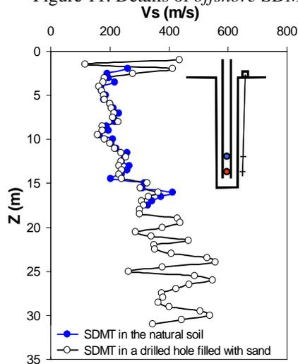
Figure 12. Comparison of  $V_S$  profiles obtained by SDMT in the natural soil and in a backfilled borehole at the site of Montescaglioso – Ginosa (Matera), Italy
