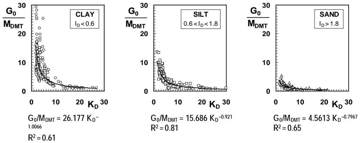
Figure 6. Ratio  $G_0/M_{DMT}$  vs.  $K_D$  for clay, silt and sand (Marchetti et al. 2008)
