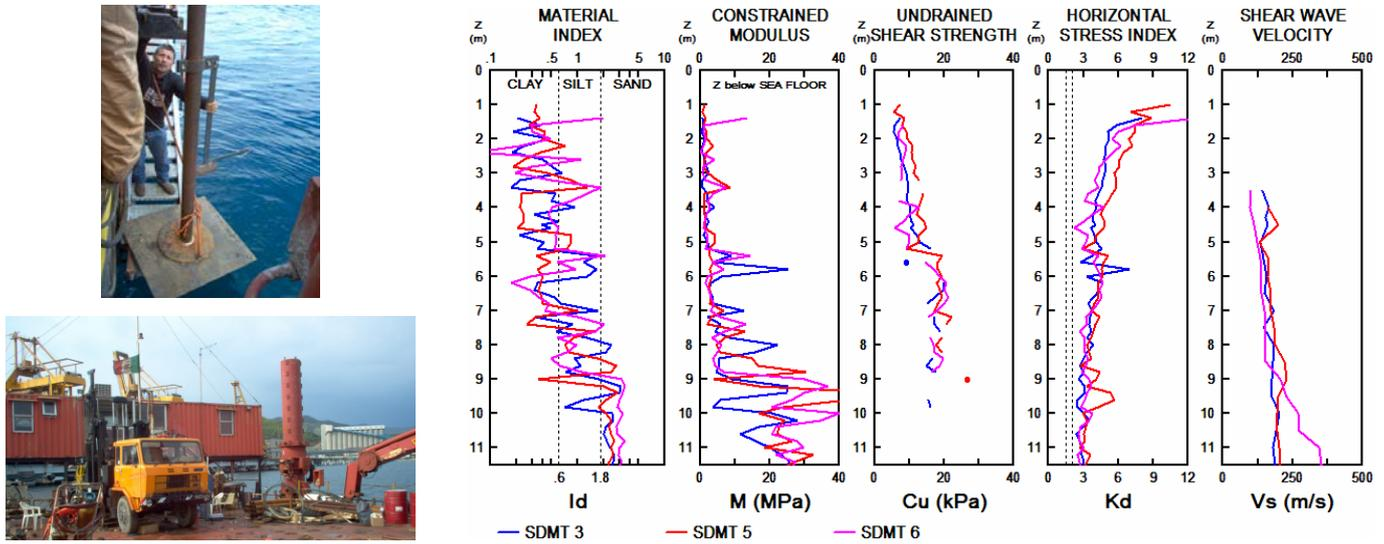
Figure 11. Details of offshore SDMT investigations and test profiles at the site of Vado Ligure (Savona), Italy
