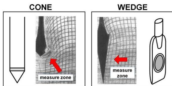
Figure 5. Distortions in clay: cone vs wedge
