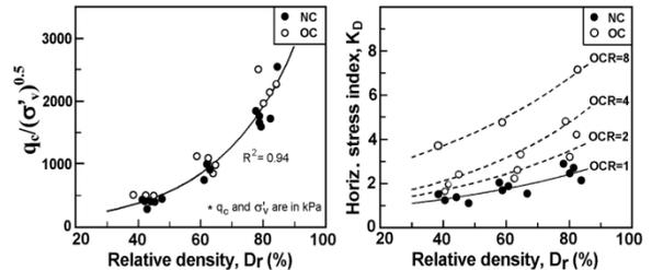
Figure 4. CPT and DMT sensitivity to stress history
