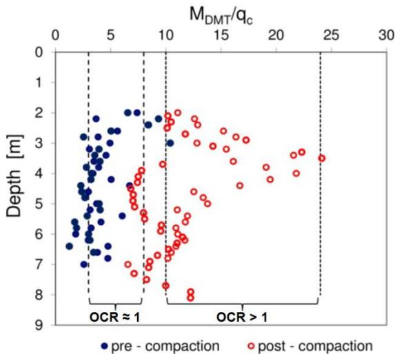
Figure 7.  $M_{DMT}/q_c$  before and after compaction
