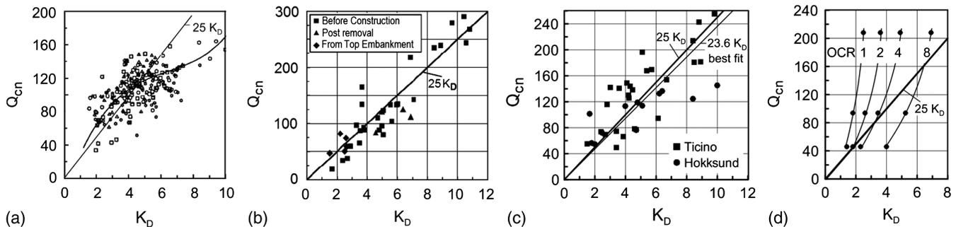
Fig. 5.  $K_D$ - $Q_{cn}$  relations: (a) from five Taiwan sand sites [reprinted from Engineering Geology, Vol. 103, No. 1-2, Pai-Hsiang Tsai, Der-Her Lee, Gordon Tung-Chin Kung, C. Hsein Juang, "Simplified DMT-based methods for evaluating liquefaction resistance of soils", pp. 13-22, Copyright (2009), with permission from Elsevier]; (b) from Treporti research site; (c) from calibration chamber results (data from Baldi et al. 1986); (d) derived from Fig. 1
