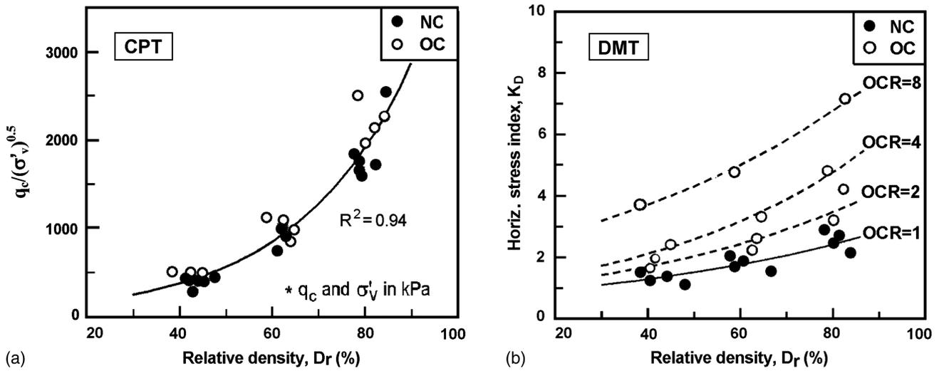
**Fig. 1.** Sensitivity of CPT and DMT to stress history: (a) CPT; (b) DMT (Reprinted from Engineering Geology, Vol. 117, No. 3-4, Moon-Joo Lee, Sung-Kun Choi, Min-Tae Kim, Woojin Lee, "Effect of stress history on CPT and DMT results in sand", pp. 259-265, Copyright (2011), with permission from Elsevier)
