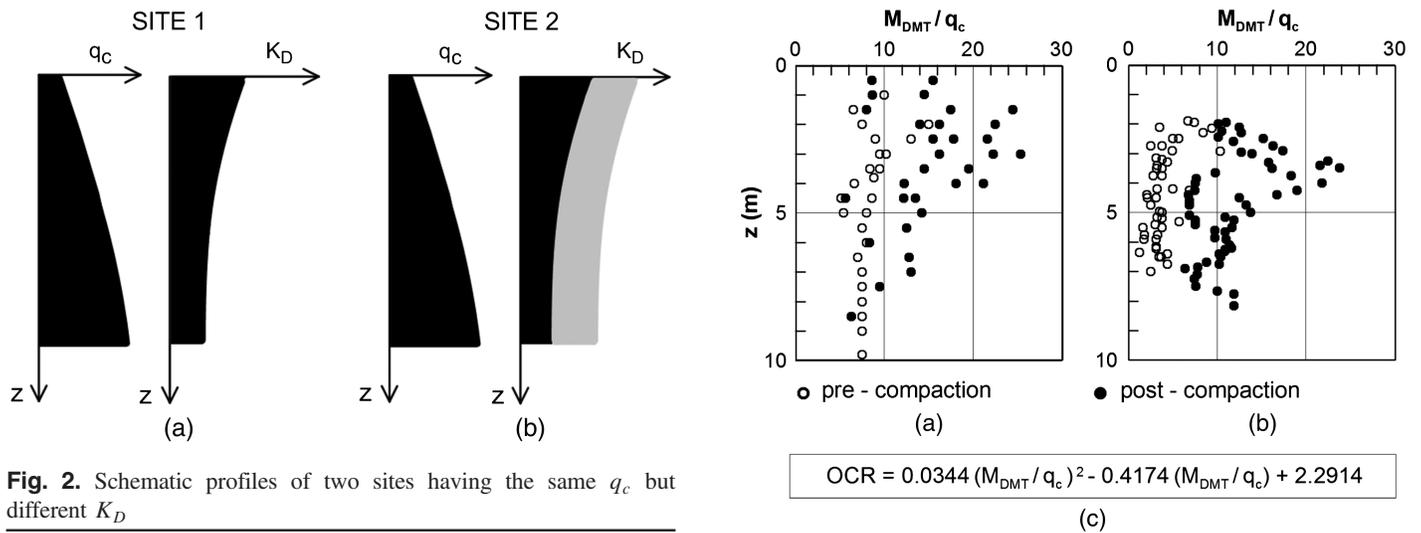
**Fig. 2.** Schematic profiles of two sites having the same  $q_c$  but different  $K_D$
