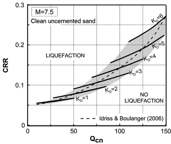
Fig. 4. Chart for estimating CRR in clean sand based on  $Q_{cn}$  and  $K_D$
