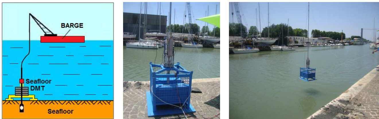
Fig. 11 Seafloor Dilatometer for executing DMT or SDMT from the seafloor
