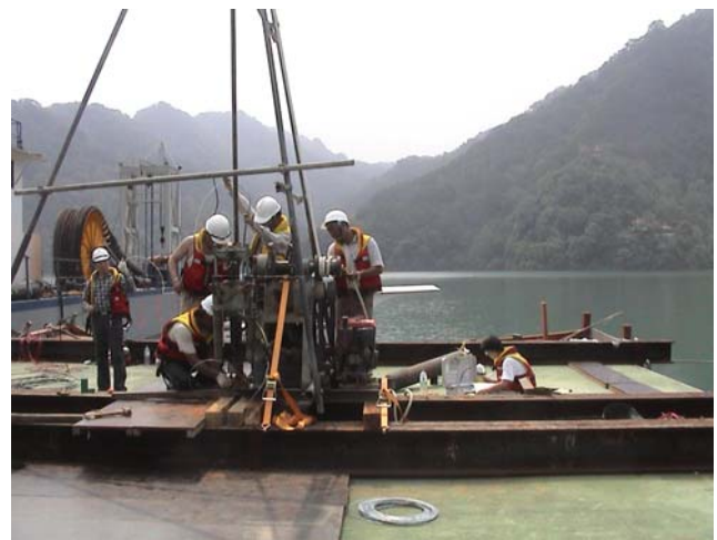
Figure 8. Operation of TDR/DMT from a barge.
