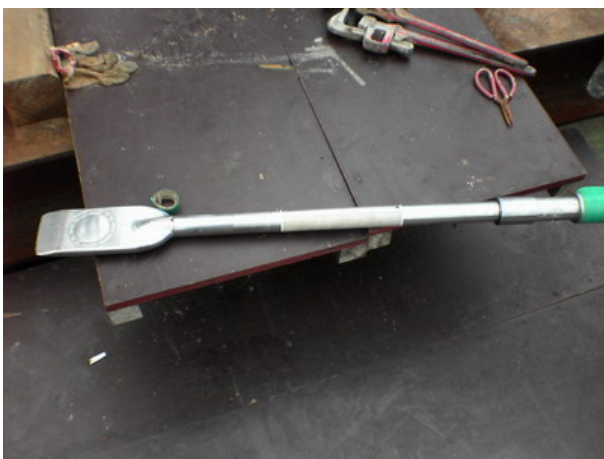
Figure 7. The TDR/DMT probe.
