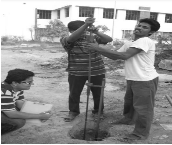
Photo.5 Field CBR by DCP method
