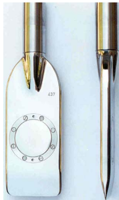
Fig. 1. The flat dilatometer - Front and side view
