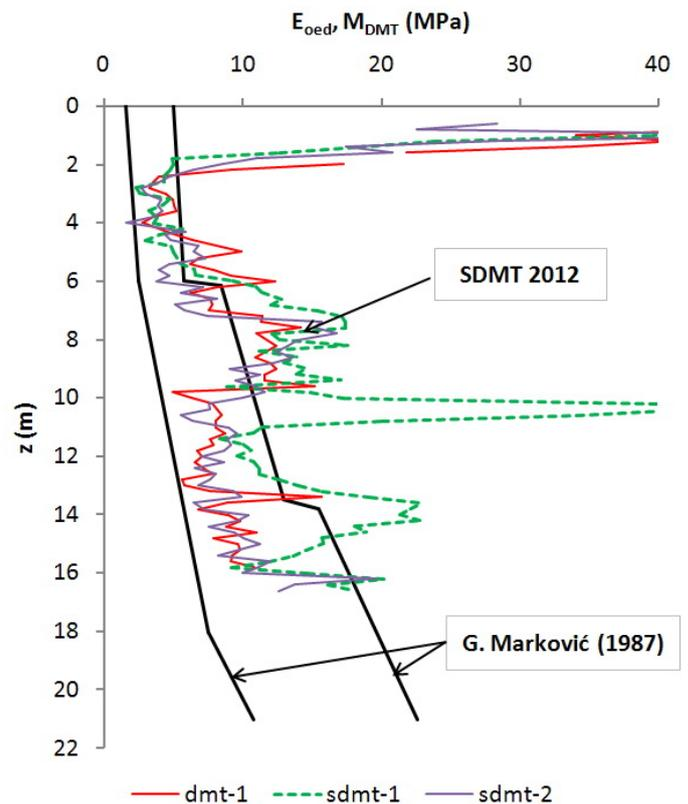
Fig. 6. Comparison of  $E_{oed}$  and  $M_{DMT}$  for Zemun loess
