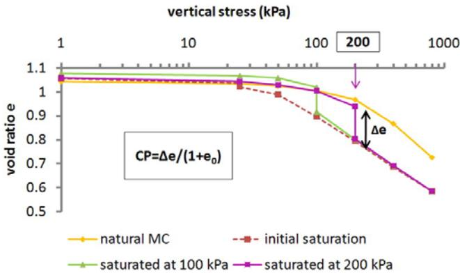
Fig 2. Oedometer test results for „Zemun loess”-first loess horizon
