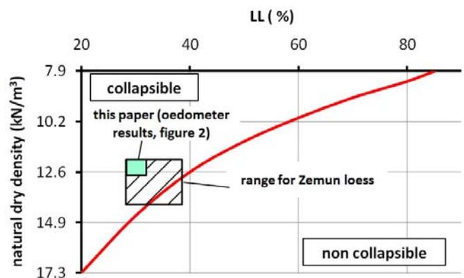
Fig. 1. Criterion for identification of collapsible soils (NAVFAC 1986)
