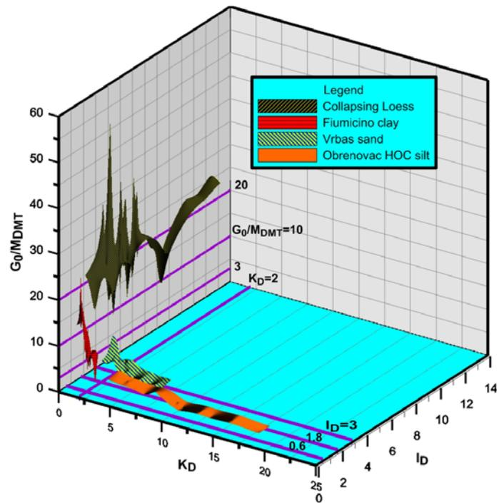
Fig. 7. 3D surface diagram showing relation of collapsible loess to „normal” soil types
