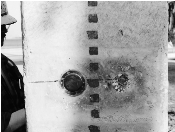
Fig. 4. DMT cell (L) and piezometer (R) on SBZ pile
