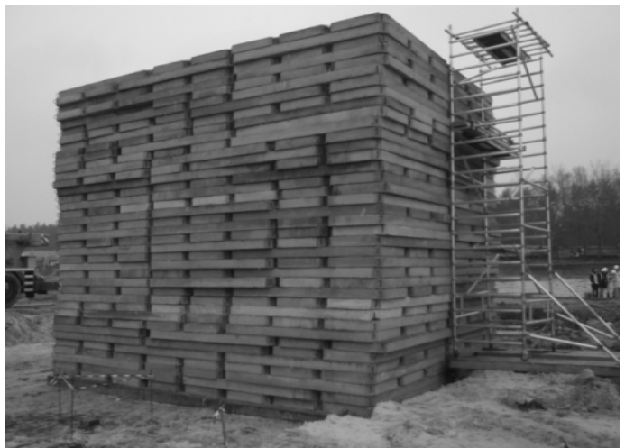
Fig. 7. View of the load structure after laying on the plate (10x10m), height of the ca 6 m.
