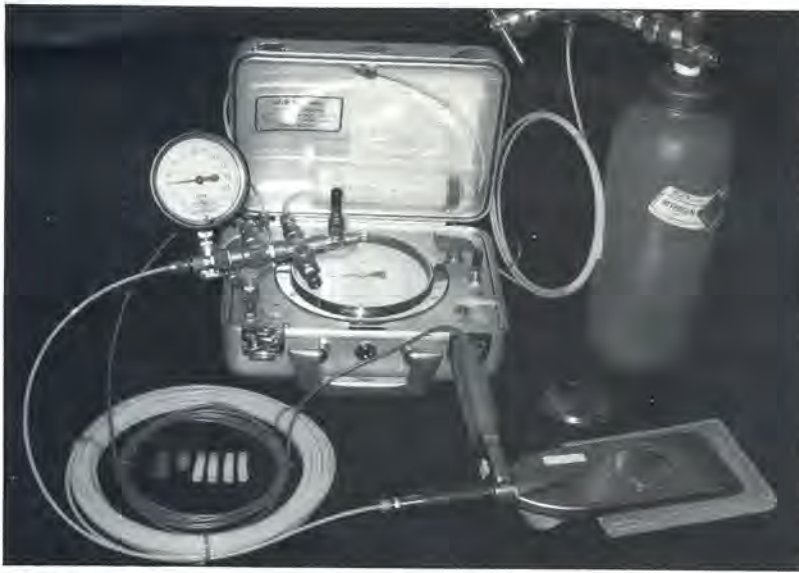
DMT equipment showing control and readout box, blade and membrane, the pneumatic-electric cable and a tank source of gas pressure.
