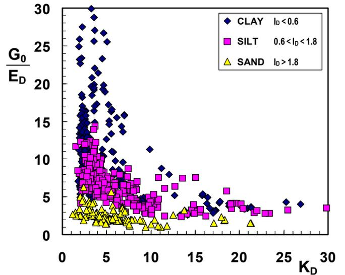
Figure 6. Ratio  $G_0/E_D$  vs.  $K_D$  for various soil types
