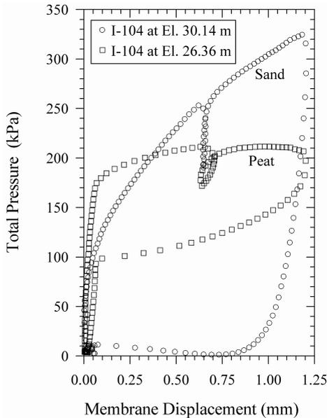
Figure 3. Typical pre-compaction IDMT tests in sand and in organic soil
