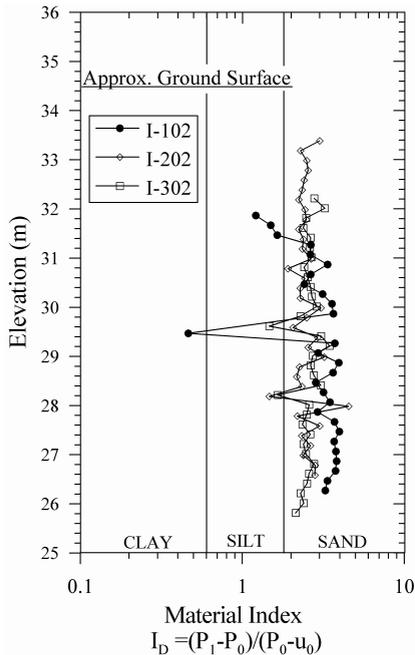
Figure 8.  $I_D$  values estimated from IDMT tests near Sta. 156
