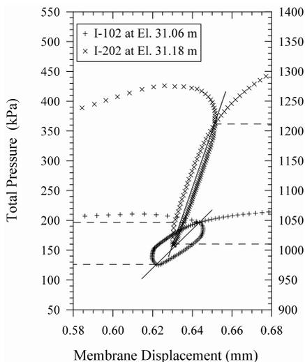
Figure 6. Pre- and post-DDC IDMT unload-reload loops
