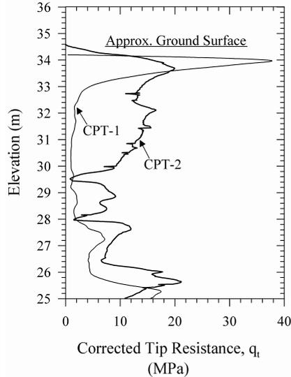
Figure 9.  $q_t$  values from CPT tests near Sta. 156
