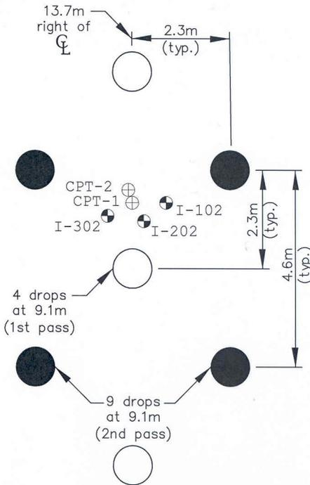
Figure 2. Details of Compaction Near IDMT Soundings
