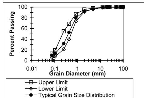
Figure 1. Grain Size Distribution of Hydraulic Fill Material
