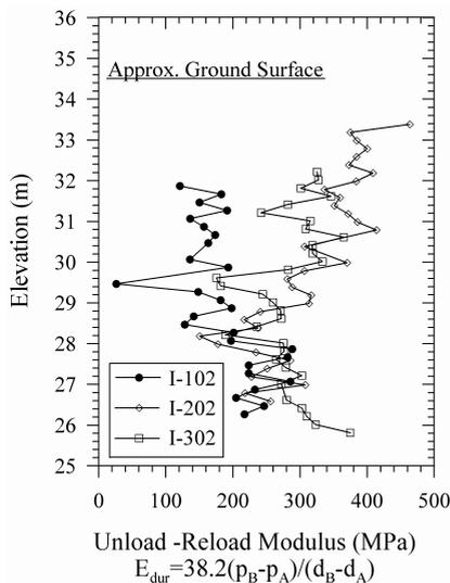
Figure 7. Profiles of unload-reload modulus,  $E_{dur}$
