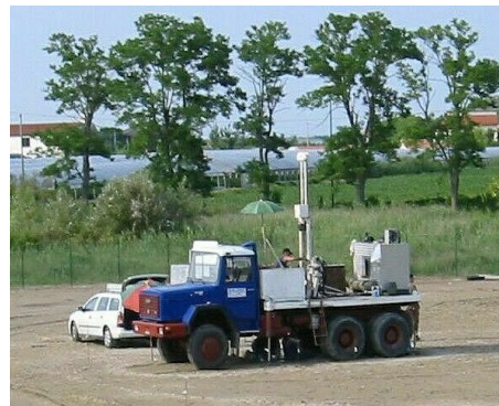
Figure 1. Cone rig used to advance the SCPTu and SDMTs.
