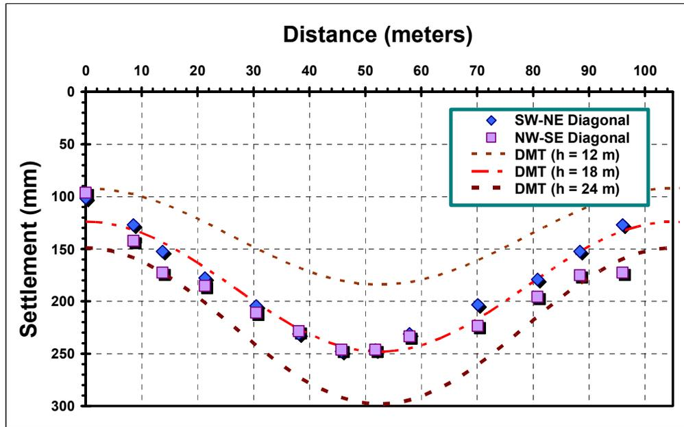
Figure 9. DMT-Calculated versus Measured Settlements for Dorm B Mat Foundation over Selected Finite Compressible Layer Thicknesses. Note: Homogeneous soil modulus  $E_s = 8.5 \text{ MPa}$  and  $q = 150 \text{ kPa}$ .
