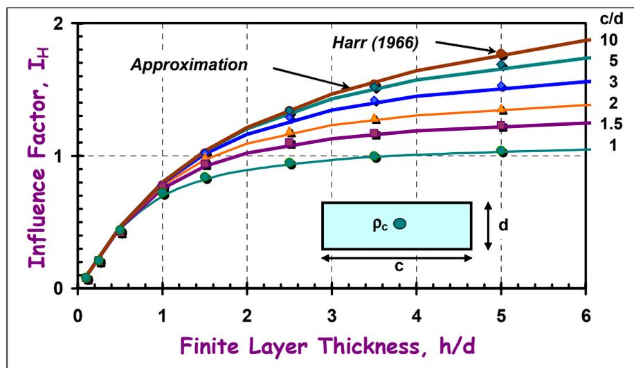
Figure 8. Displacement Influence Factors for Flexible Rectangular Foundation Resting on Finite Homogeneous Layer and Smooth Subsurface Interface ( $\nu = 0$ ). Approximate numerical integration solution (after Mayne & Poulos, 1999) compared with closed-form elastic solution (Harr 1966)
