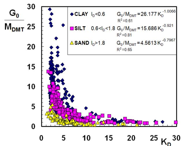
Fig. 5 Ratio  $G_0 / M_{DMT}$  vs.  $K_D$  (OCR) for various soil types [8]. It can provide estimates of  $G_0$  (and  $V_S$ ) from the results of the "mechanical" DMT
