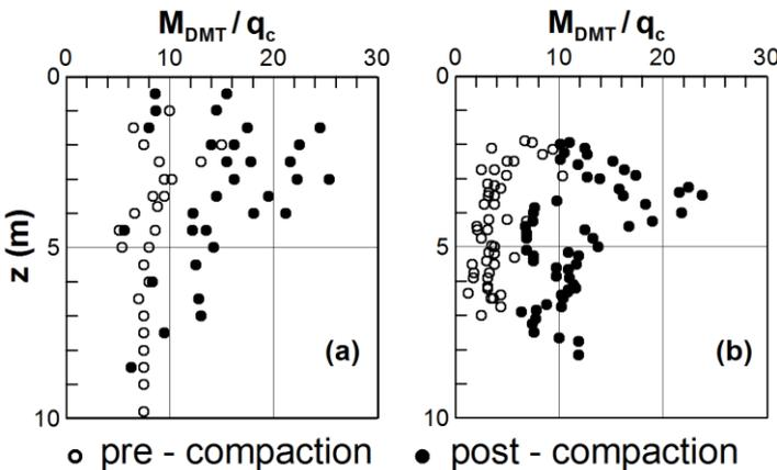
**Fig. 10**  $M_{DMT}/q_c$  ratio before/ after compaction. (a) Jendebay (1992) [12] (b) Balachowski and Kurek (2015 [19])
