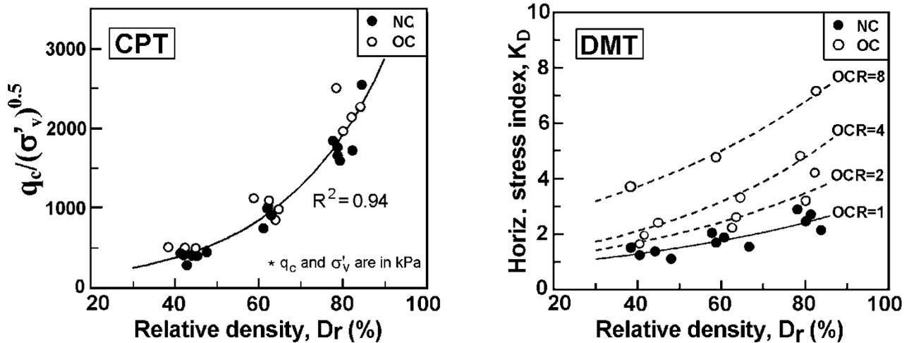
Fig. 4 Sensitivity of CPT and DMT to Stress History (Lee et al. 2011 [13])
