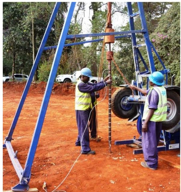
**Fig. 7** DMT blade advanced by an SPT rig
