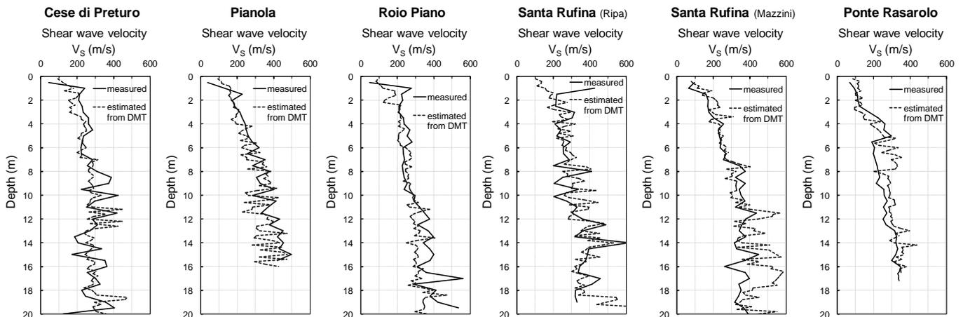
**Fig. 6** Comparison of profiles of  $V_S$  measured by SDMT and estimated from mechanical DMT data, by use of the correlations in Fig. 5, at six sites in the area of L'Aquila (Monaco at al. 2013 [14])
