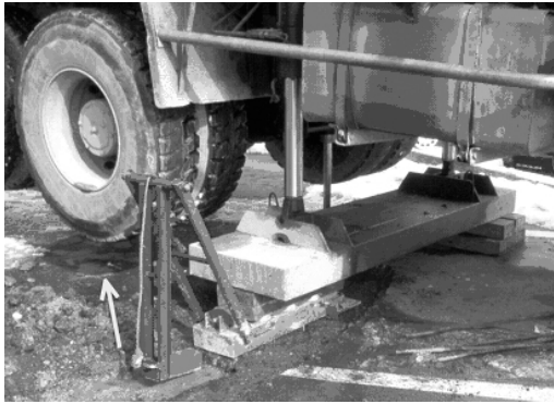
FIG. 2. Shear wave source at the surface
