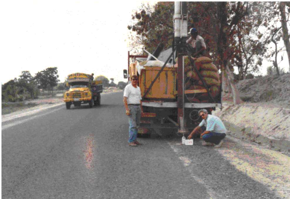
Fig. 3 – Truck mounted penetrometer used for pushing the dilatometer blade
