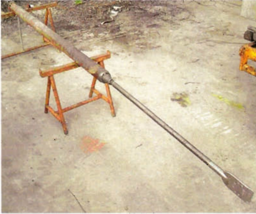
Figure 1. Wire-line dilatometer with nitrogen tank and computer control unit inside large steel housing.
