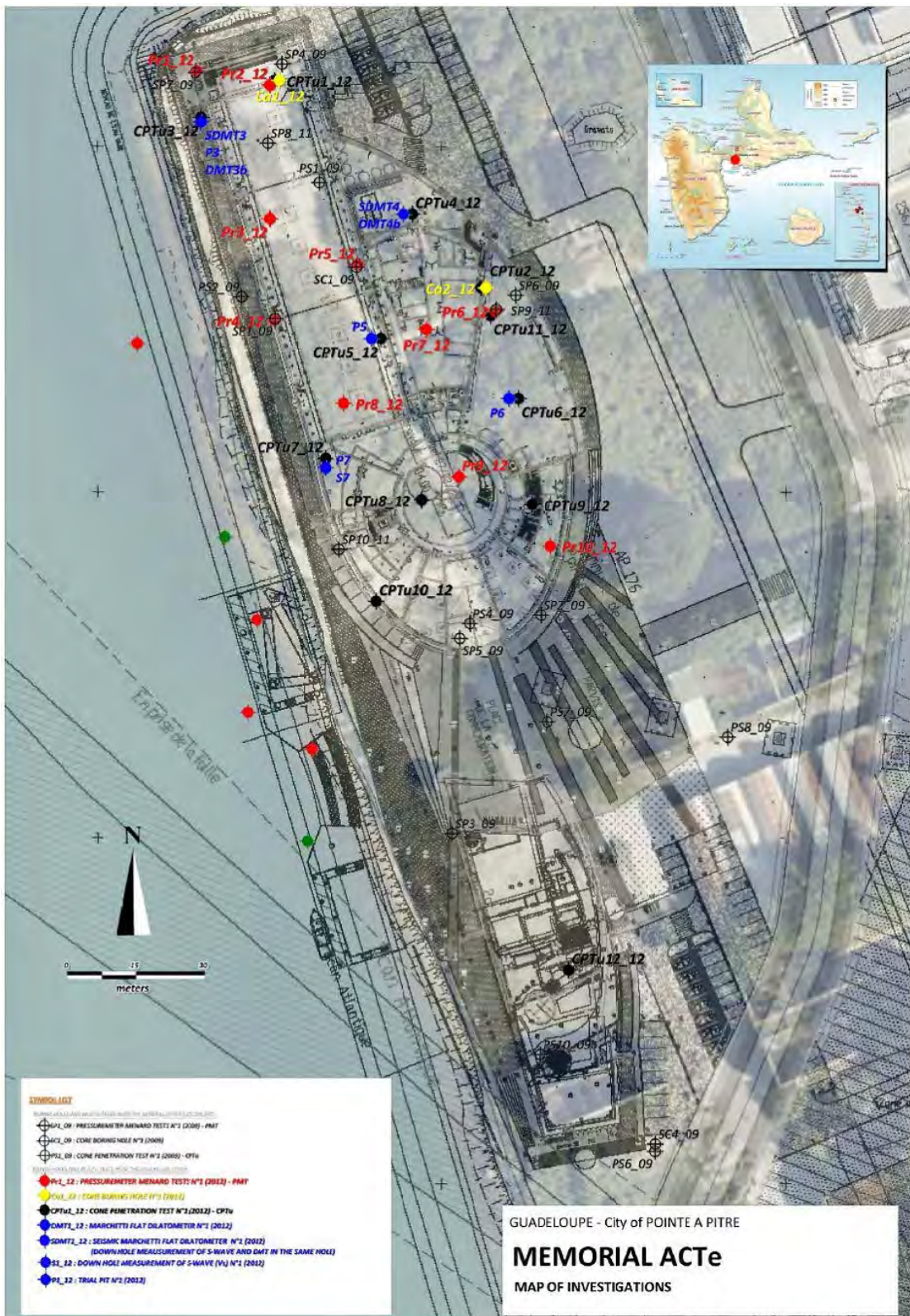
Figure 3. MACTe: plan of the geotechnical investigations.
