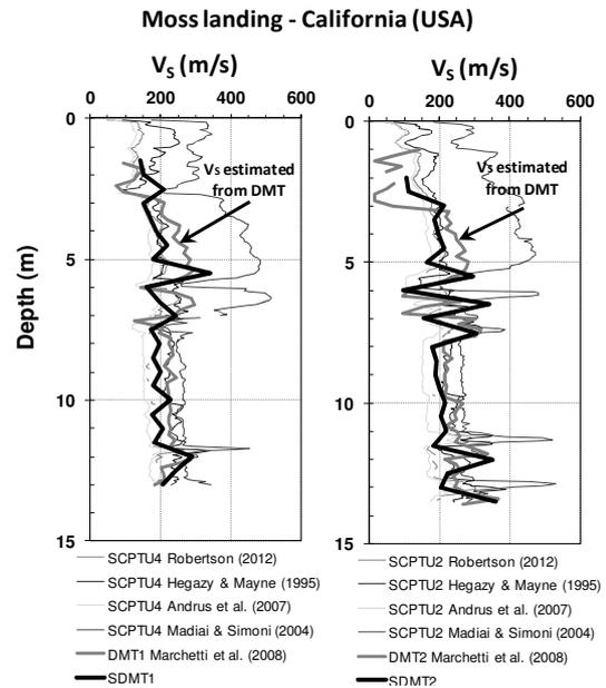
Figure 3. Comparison of  $V_s$  measured by SDMT or SCPT and estimated from CPT and DMT data at Moss Landing - California (USA).
