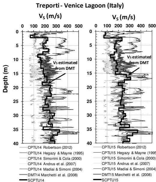
Figure 2. Comparison of  $V_s$  measured by SCPT and estimated from CPT and DMT data at Treporti-Venice Lagoon (Italy) - Before construction.
