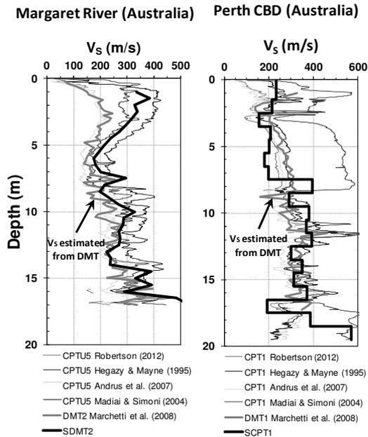
Figure 5. Comparison of  $V_S$  measured by SDMT or SCPT and estimated from CPT and DMT data at Margaret River and Perth CBD (Western Australia).
