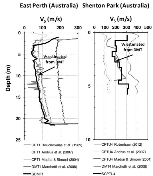
Figure 4. Comparison of  $V_s$  measured by SDMT or SCPT and estimated from CPT and DMT data at East Perth and Shenton Park (Western Australia).
