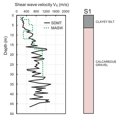
Figure 13. Profile of  $V_s$  measured by SDMT in a back-filled borehole,  $V_s$  measured by MASW (IAMC-CNR, MS-AQ Working Group 2010) and schematic soil profile at the site of Via Solaria (Cansatessa), L'Aquila.
