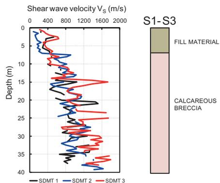
Figure 8. Profiles of  $V_s$  measured by SDMT in 3 back-filled boreholes and schematic soil profile at the site of Palazzo Carli, L'Aquila.
