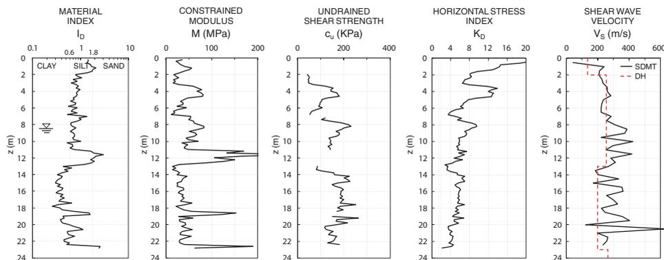
Figure 4. SDMT results at the site of Cese di Preturo (C.A.S.E. Project), L'Aquila. *On the right:* Comparison of profiles of  $V_s$  from SDMT and Down-Hole (Polo Geologico, MS-AQ Working Group 2010).
