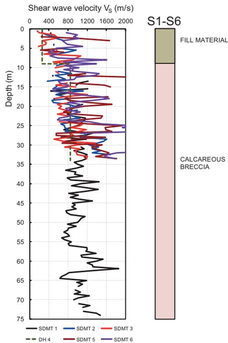
Figure 7. Profiles of  $V_s$  measured by SDMT in 5 back-filled boreholes,  $V_s$  measured by Down-Hole and schematic soil profile at the site of Palazzo Camponeschi, L'Aquila.
