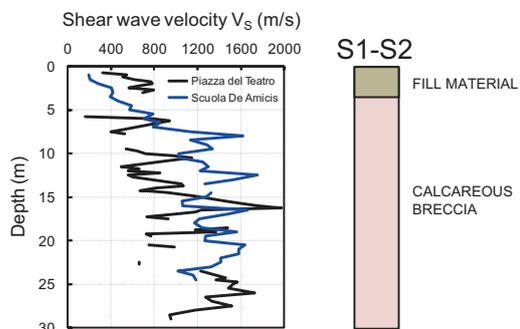
Figure 10. Profile of  $V_s$  measured by SDMT in 2 back-filled borehole and schematic soil profile at the site of Piazza del Teatro—Scuola De Amicis, L'Aquila.
