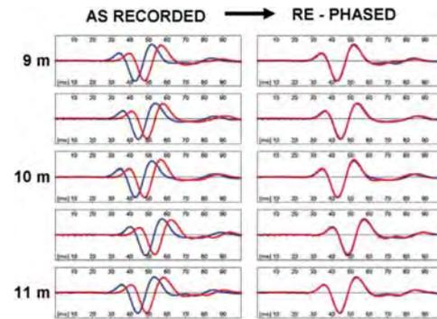
Figure 2. Example of seismograms obtained by SDMT (test site of Fucino, Marchetti et al. 2008).
