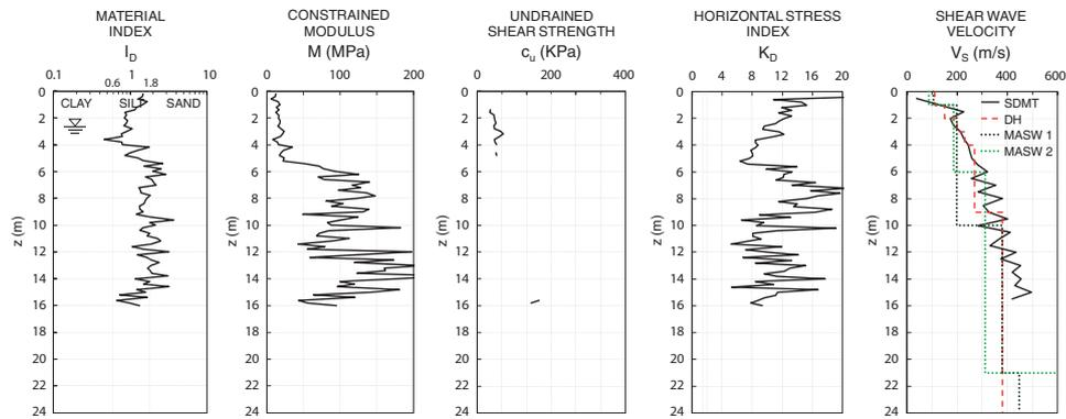
Figure 6. SDMT results at the site of Pianola (C.A.S.E. Project), L'Aquila. *On the right*: Comparison of profiles of  $V_s$  from SDMT, Down-Hole (Polo Geologico) and MASW (Politecnico di Torino, MS-AQ Working Group 2010).
