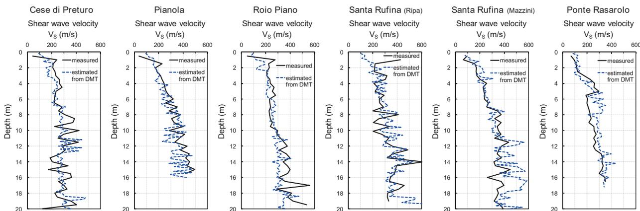
Figure 16. Comparison of profiles of  $V_s$  measured by SDMT and estimated from mechanical DMT data, by use of the correlations in Figure 15, at six sites in the area of L'Aquila.
