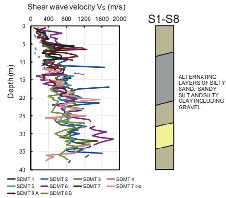
Figure 12. Profiles of  $V_s$  measured by SDMT in 8 backfilled boreholes and schematic soil profile at the site of San Salvatore Hospital (Coppito), L'Aquila.
