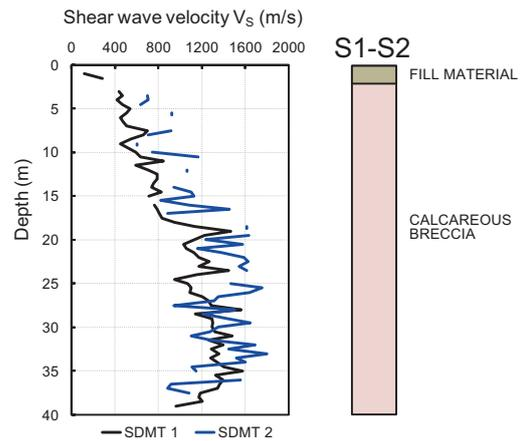
Figure 9. Profile of  $V_s$  measured by SDMT in 2 back-filled borehole and schematic soil profile at the site of Palazzo Margherita, L'Aquila.
