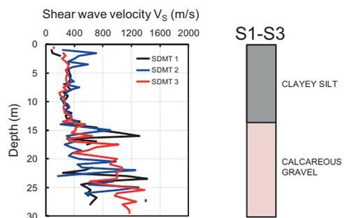
Figure 14. Profile of  $V_s$  measured by SDMT in 3 back-filled boreholes and schematic soil profile at the site of Via Sila Persichelli (Pettino), L'Aquila.
