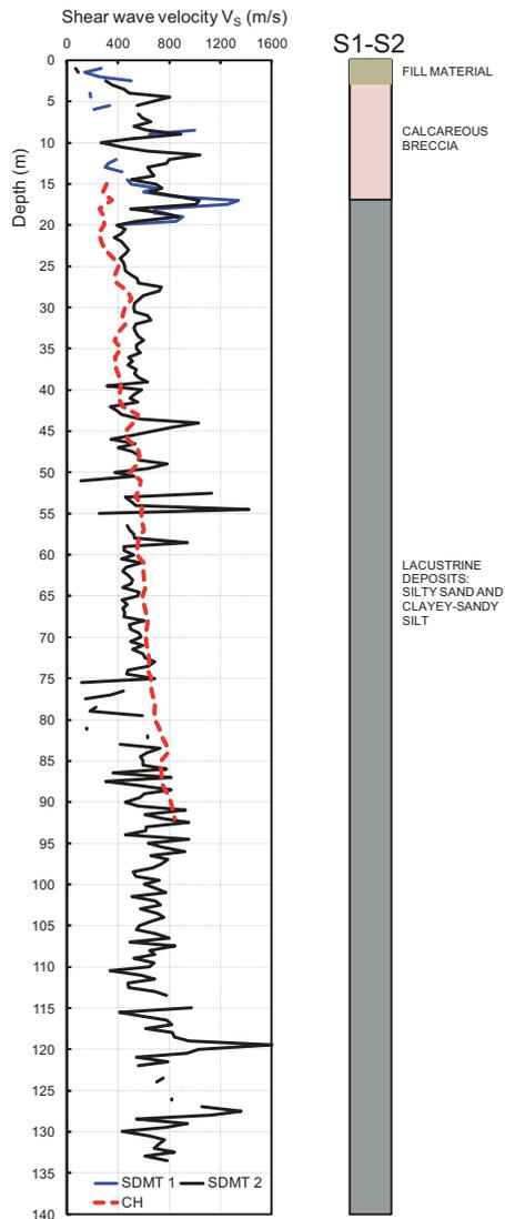
Figure 11. Profiles of  $V_s$  measured by SDMT in 2 back-filled boreholes,  $V_s$  measured by Cross-Hole in a nearby site (Cardarelli & Cercato 2010) and schematic soil profile at the site of Fontana 99 Cannelle, L'Aquila.
