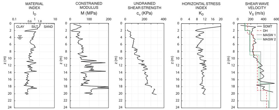
Figure 5. SDMT results at the site of Roio Piano (C.A.S.E. Project), L'Aquila. *On the right*: Comparison of profiles of  $V_s$  from SDMT, Down-Hole (Polo Geologico) and MASW (Politecnico di Torino, MS-AQ Working Group 2010).
