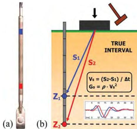
Figure 1. Seismic dilatometer test: (a) DMT blade and seismic module; (b) Schematic test layout.
