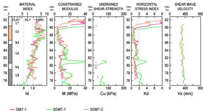
Fig. 4. SDMT/DMT results for Zemun loess
